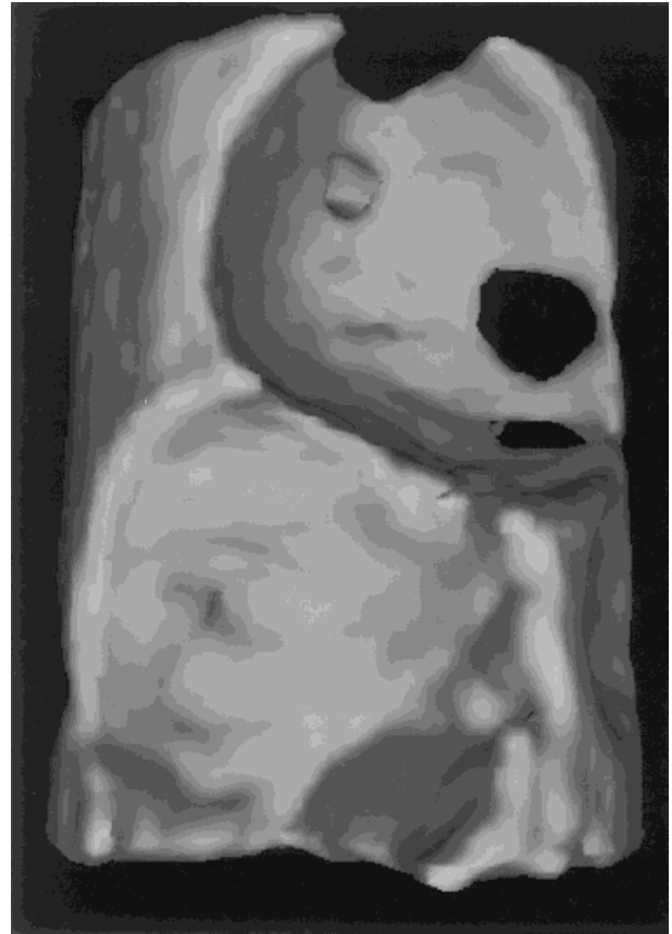
Figure 4 A three-dimensional rendering of a 1-mm-diameter cylinder through the center of the foam shown in Figure 3. Circular openings connect adjacent pores.
